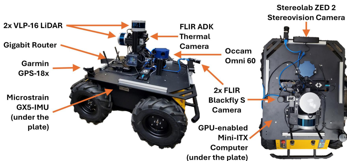
Figure 3. Cypector (mobile robot) and its multi-modal sensors and other equipment.
